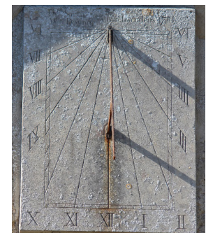
9.15 am BST Thursday 25th June 2020. Adjusting to 8.15 am GMT it shows the dial has been calibrated well. The gnomon shadow (top) had just appeared as the sun emerged south of the plane of the sundial face
